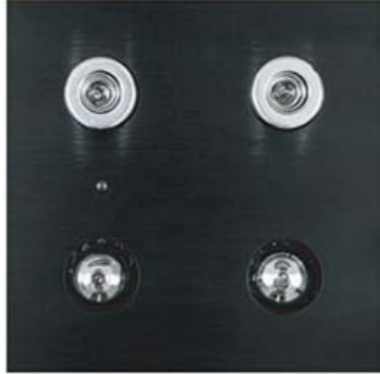
Two cascaded preamplifiers
